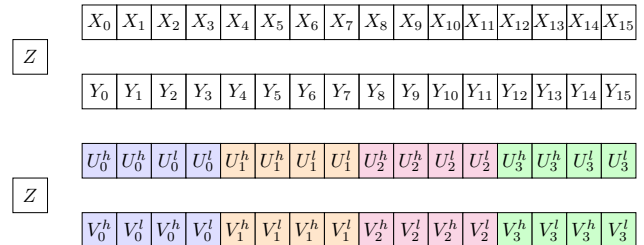
Fig. 1. FP16 dot product of size 16 R = Z + \sum X_i \times Y_i (top), used as an FP32 dot product of size 4 (bottom).
